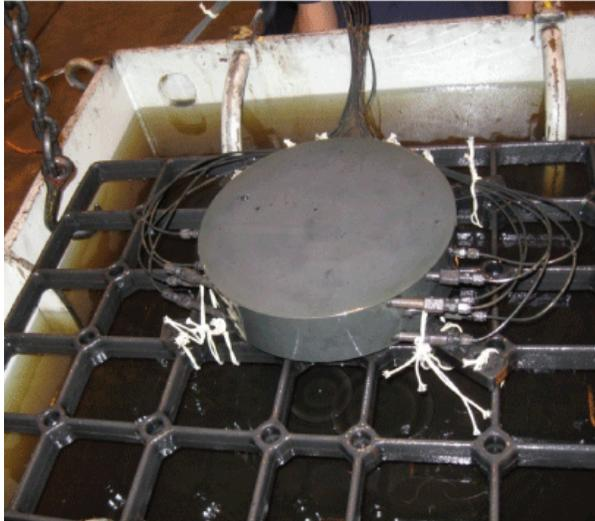
**Figure 4.** The actual test pancake with the 11 thermocouples embedded into it. The pancake sits on the quenching rack above the oil bath. Leads are seen coming from the thermocouples for data acquisition during quenching. The pancake has thermocouples located throughout the volume.
